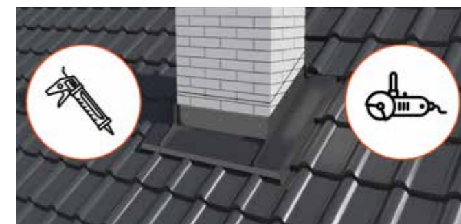
Fig. 21 Chimney cut before installation of top flashings.
