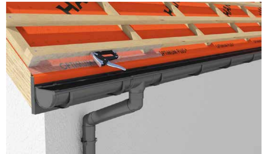
Fig. 9 Installation of perforated mesh to protect the roof eaves from insects and debris.
