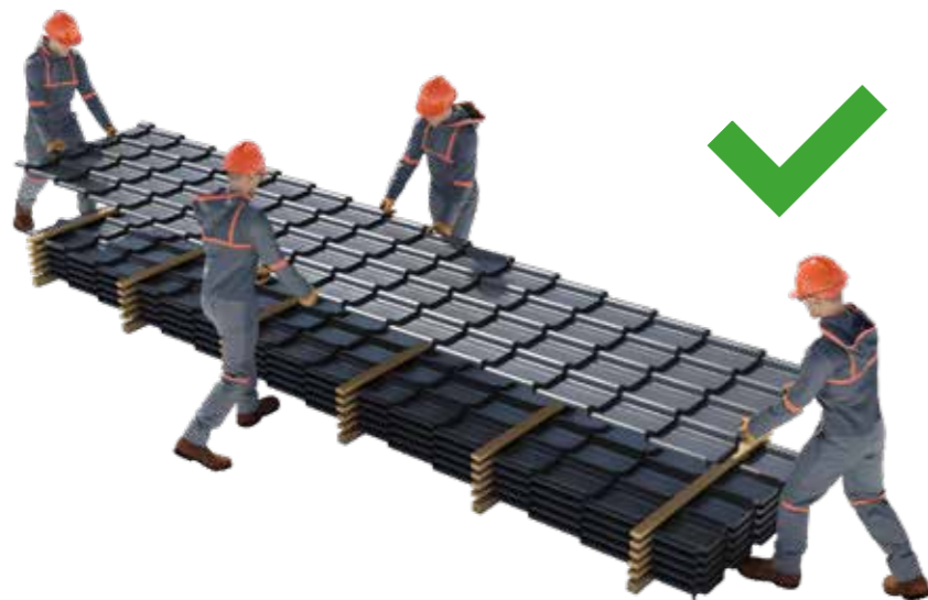
Fig. 2 Correct way of transporting steel roofing tiles.
