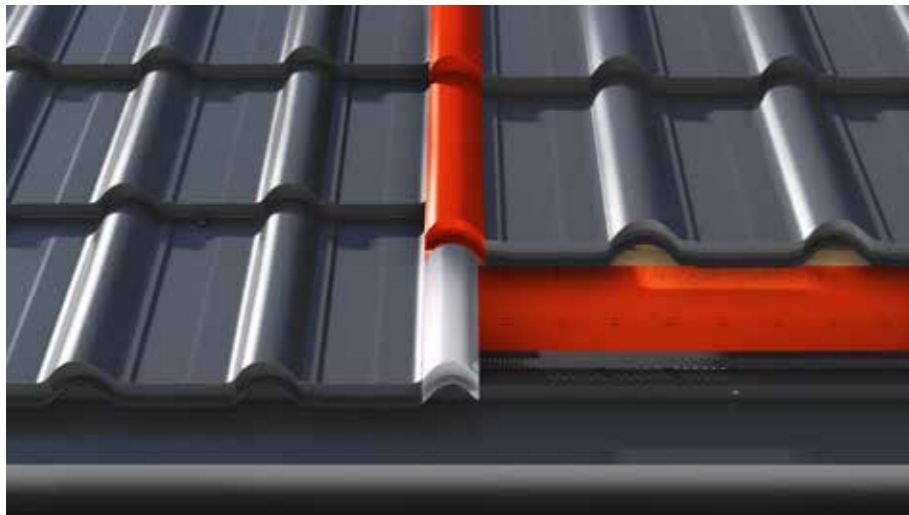
Fig. 15 Longitudinal overlap when joining roofing sheets.
