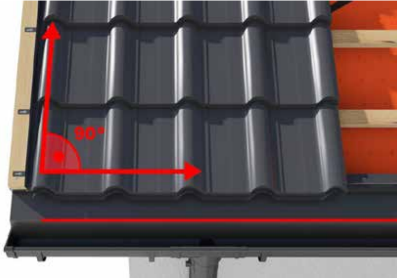
Fig. 14 Installation of the first sheet at a 90 degree angle to the eaves.
