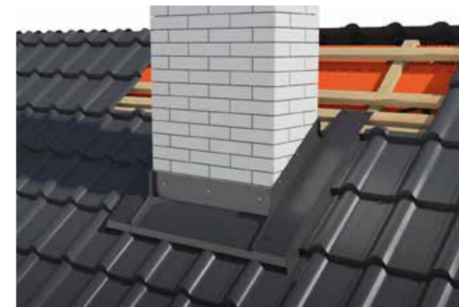
Fig. 20 Installation of chimney flashing - front and sides.
