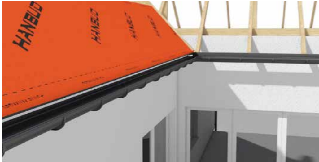
Fig. 6 Membrane distribution on the slope surface.
