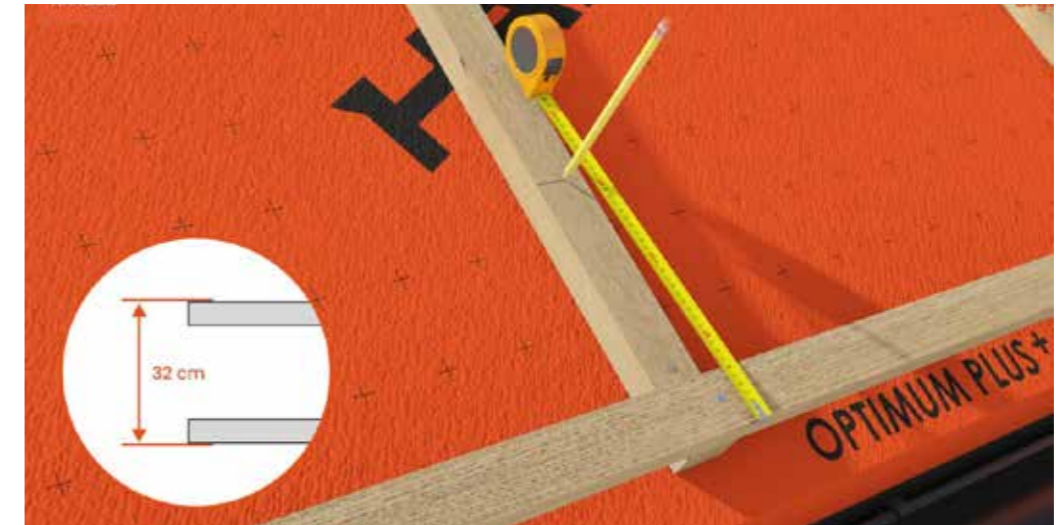
Fig. 8 Layout of battens on the roof slope.
