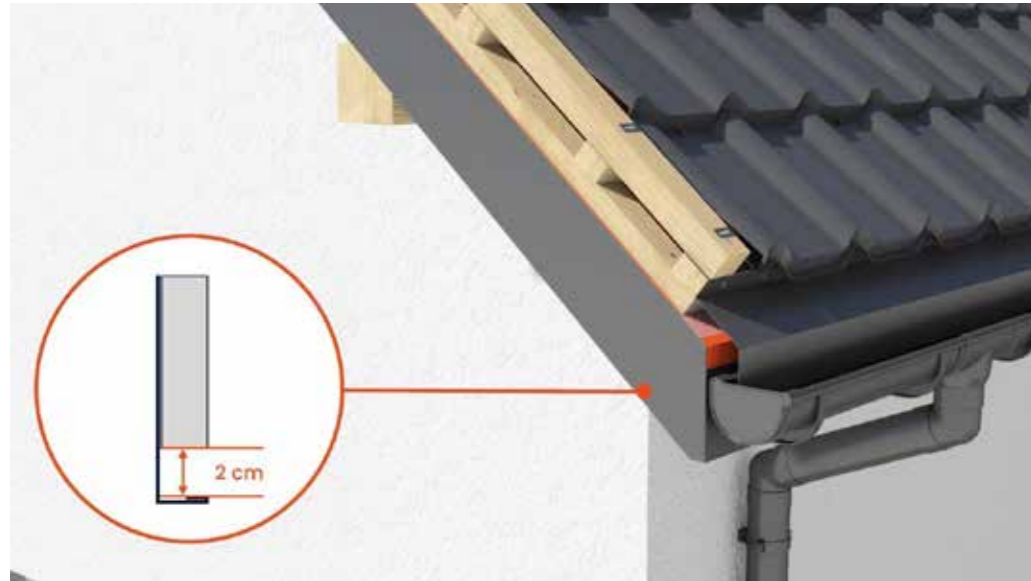
Fig. 18 Assembling the wind brace with a 2 cm overlap.
